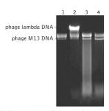
Action of DSN on ss DNA of phage M13 and ds DNA of phage lambda.
