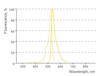
PhiYFP normalized excitation (thin line) and emission (thick line) spectra. Complete PhiYFP spectra in Excel format can be downloaded from the Evrogen Web site at http://www.evrogen.com
